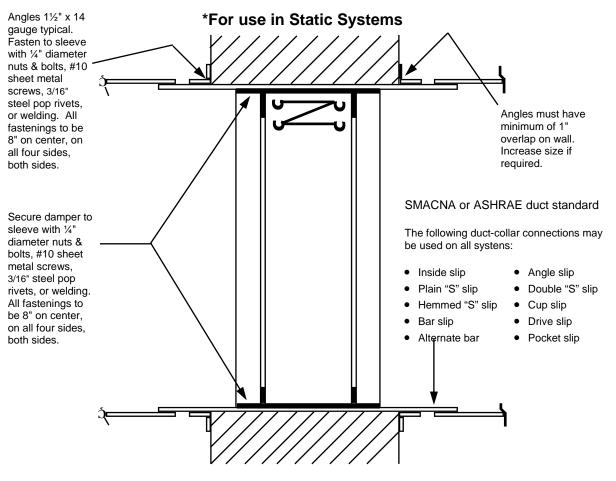
\*These instructions are for mounting the damper in a masonry or gypsum wallboard wall or partition, or a concrete floor.
